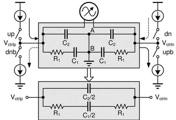
Fig. 7. Circuit diagram of the differential-mode LPF.
