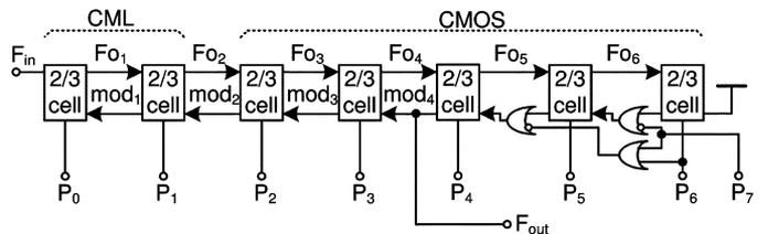
Fig. 8. Circuit diagram of the programmable cascaded divider.
