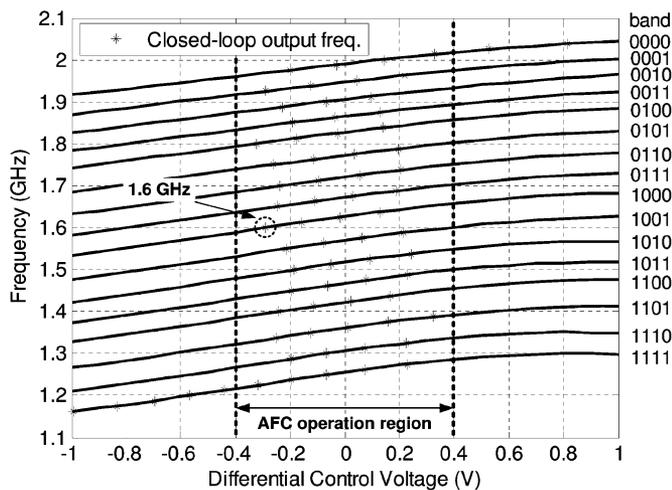
Fig. 10. Measured tuning curves of 16 sub-bands.
