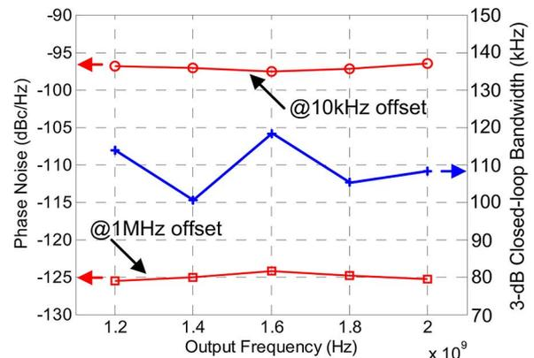
Fig. 13. Measured phase noise and 3-dB closed-loop bandwidth.
