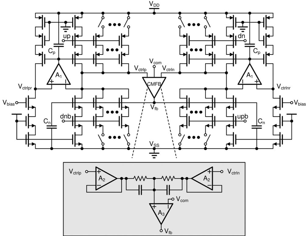
Fig. 6. Circuit diagram of the differential CP.
