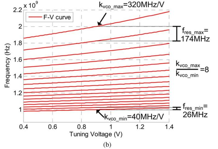
Fig. 2. Conventional topology. (a) Switching capacitor array and one varactor unit. (b)  $F$ - $V$  curve with large variations of VCO tuning gain and band step.
