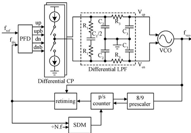
Fig. 5. Block diagram of the 2–2.4 GHz fractional-*N* frequency synthesizer.
