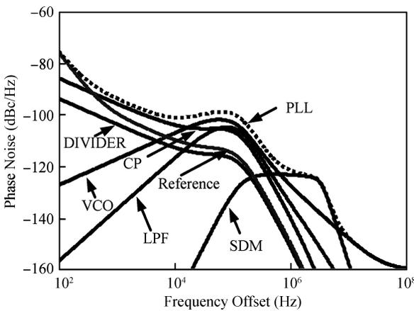
Fig. 4. PLL phase noise simulation.
