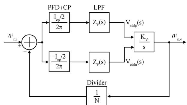
Fig. 1. Simplified block diagram for differentially-tuned frequency synthesizer.
