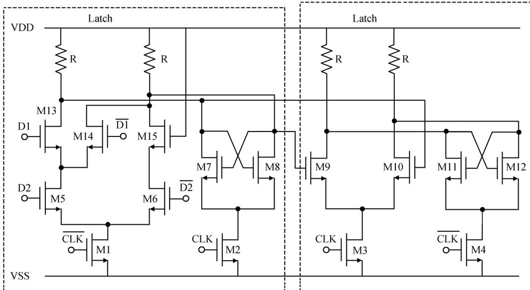
Fig. 9. "NAND" embedded CML D-flip-flop.
