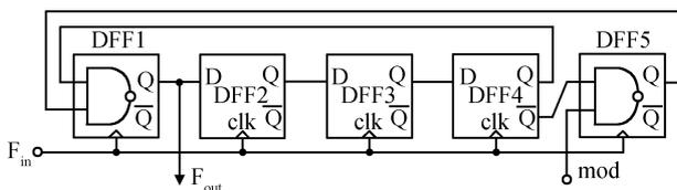
Fig. 8. High speed synchronous 8/9 prescaler diagram.
