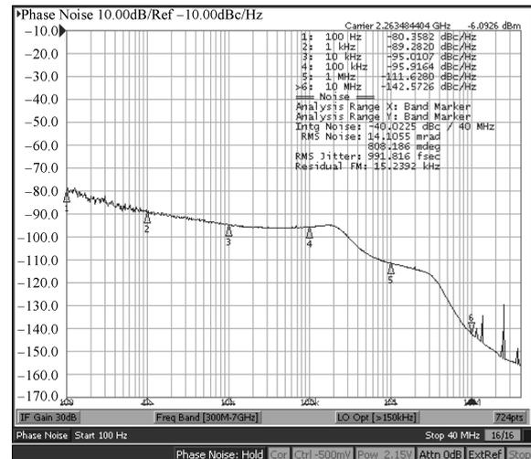
Fig. 11. Measured phase noise at an oscillation frequency of 2.26 GHz.
