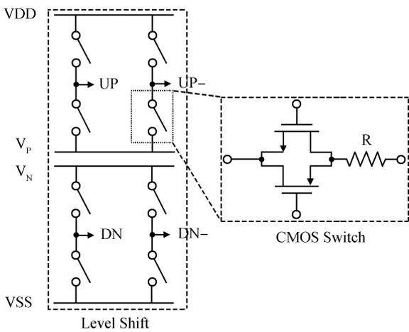
Fig. 7. Level shift and switch.
