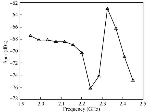
Fig. 14. Reference spurs at different output frequencies.
