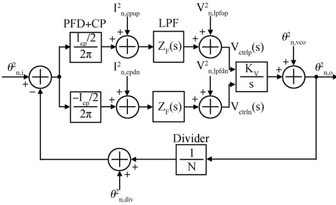
Fig. 2. Noise model for differentially-tuned frequency synthesizer.
