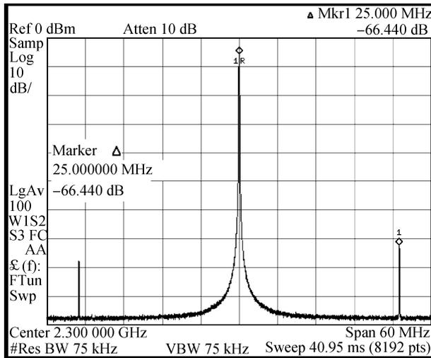
Fig. 13. Measured power spectrum density (PSD) of the oscillation amplitude at 2.3 GHz.
