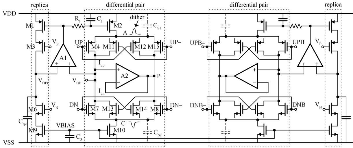
Fig. 6. Fully-differential charge pump without common-mode feedback.
