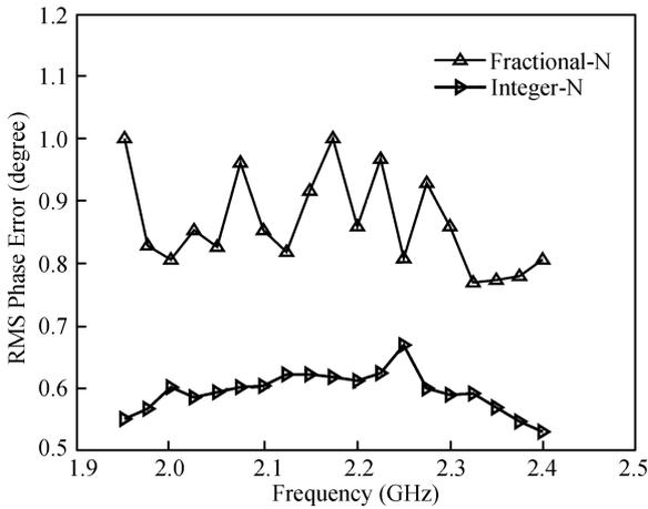
Fig. 12. RMS phase error (integrated from 100 Hz to 100 MHz).
