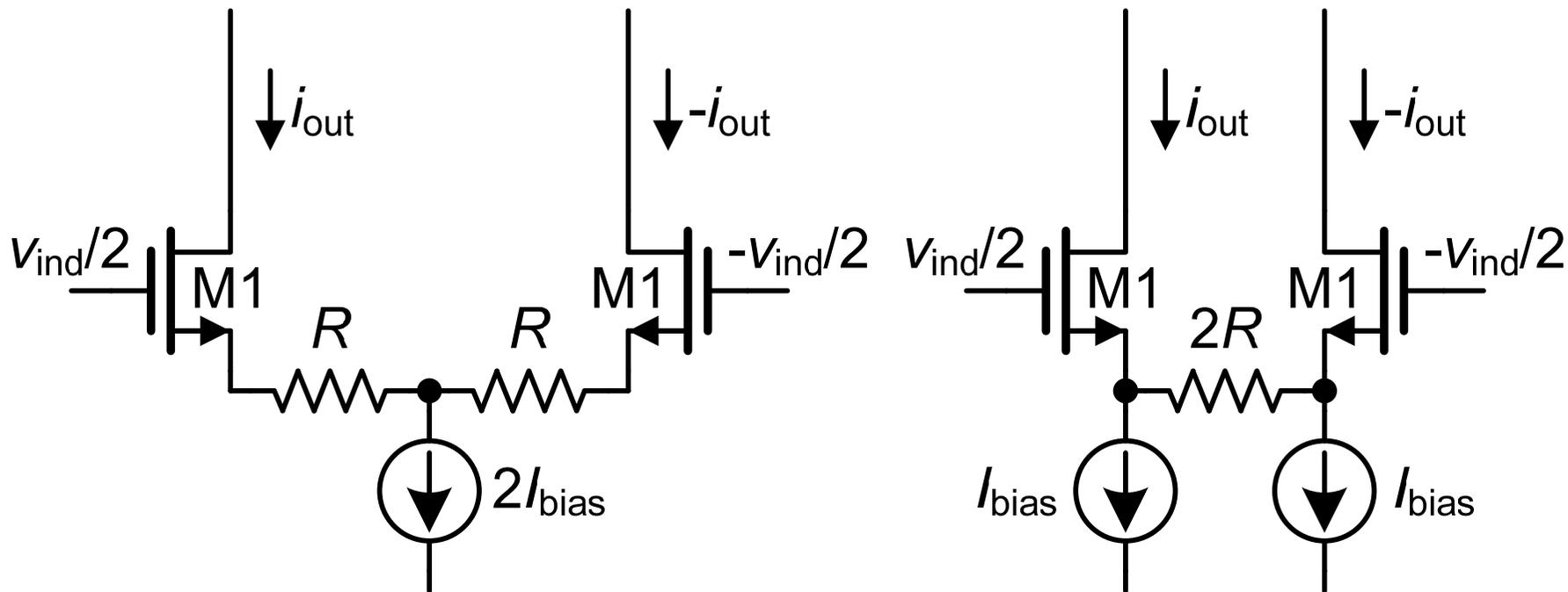
$$IP_3 \approx 3.3(V_{GS} - V_T)(1 + g_{m1}R)^{3/2} \quad HD_3 = \frac{1}{32} \frac{U^2}{(1 + g_{m1}R)^3}$$
