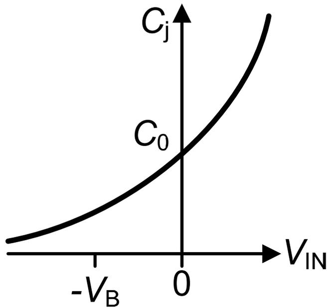
$$C_j = \frac{C_0}{\sqrt{1 - \frac{V_{IN}}{\Phi}}} \quad V_{IN} = -V_B + V_{in}$$
