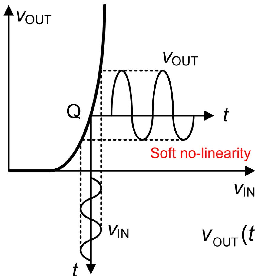
$$v_{IN}(t) \Rightarrow v_{OUT}(t)$$
