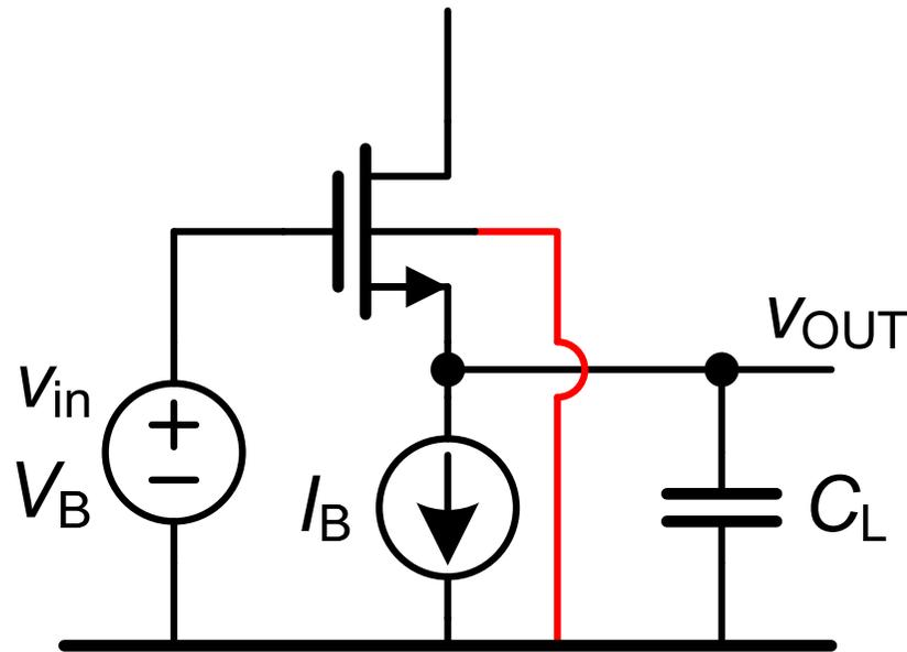
$$V_{OUT} = V_{IN} - V_{GS}$$
