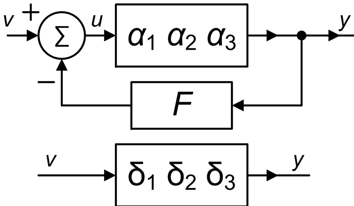
$$\left. \begin{aligned} u &= v - Fy \\ y &= \alpha_1 u + \alpha_2 u^2 + \alpha_3 u^3 \end{aligned} \right\} \text{elim. } u \left\{ \begin{aligned} \text{coeff. } v &: \delta_1 \\ \text{coeff. } v^2 &: \delta_2 \\ \text{coeff. } v^3 &: \delta_3 \end{aligned} \right. \\
