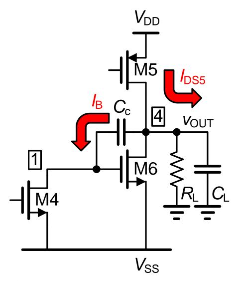
$$SR_{\text{int}} = \frac{I_{\text{B}}}{C_{\text{c}}}$$
