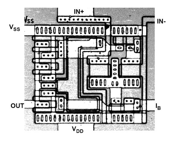
GBW = 1 MHz  $C_L = 10 \text{ pF}$  SR = 2.2 V/µs  $V_{DD} = 5 \text{ V}$   $I_{TOT} = 27 \text{ µA}$
