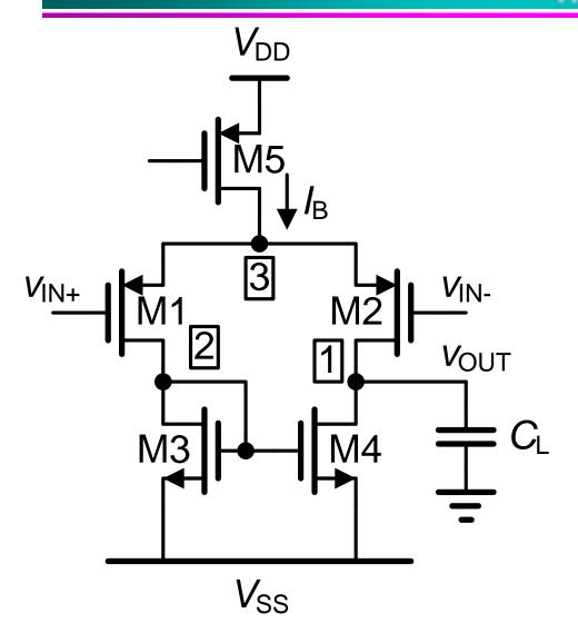
$$GBW = \frac{g_{\text{m1}}}{2\pi(C_{\text{L}} + C_{\text{n1}})}$$
