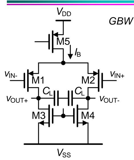
$$GBW = \frac{g_{m1}}{2\pi C_L} \qquad g_{m1} = \frac{I_B}{V_{GS1} - V_T}$$
