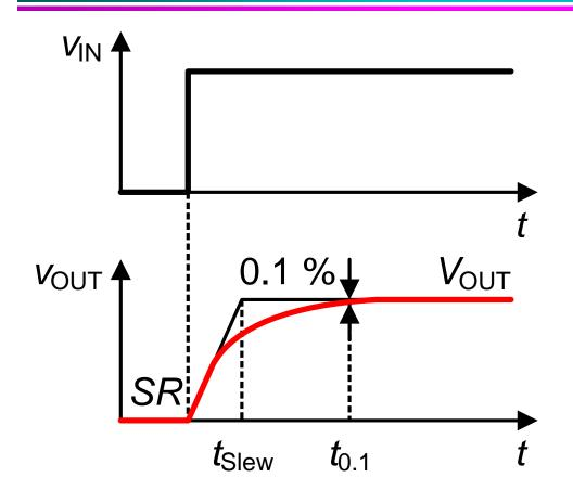
$$t_{ ext{TOT}} = t_{ ext{Slew}} + t_{0.1}$$
