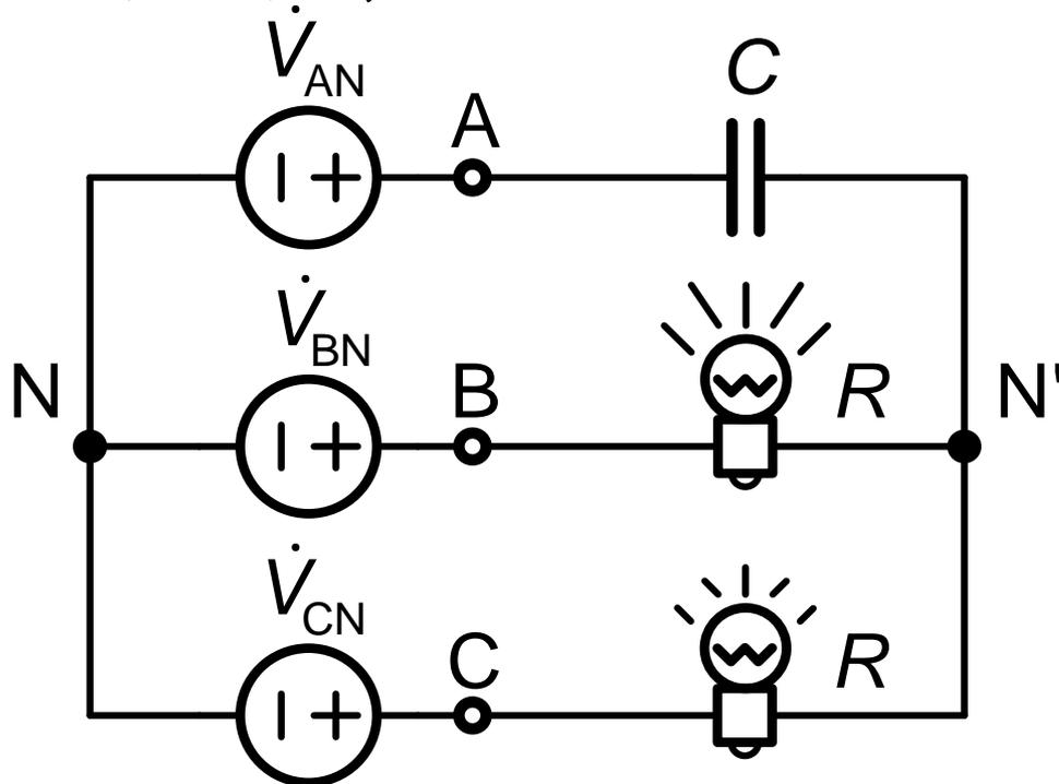
$$\begin{aligned}\dot{V}_{N'N} &= \frac{\dot{V}_{AN}/Z_A + \dot{V}_{BN}/Z_B + \dot{V}_{CN}/Z_C}{1/Z_A + 1/Z_B + 1/Z_C} \\ &= \frac{j\omega C\dot{V}_{AN} + \dot{V}_{AN}/(\alpha R) + \dot{V}_{AN}/(\alpha^2 R)}{j\omega C + 1/R + 1/R} \\ &= \frac{-1 + j3}{5} \dot{V}_{AN}\end{aligned}$$
